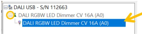
For each address the group membership, scene values and DALI-parameters can be set. In Colour&Dim operating mode, all values assigned to channel 2 are representing colours.
