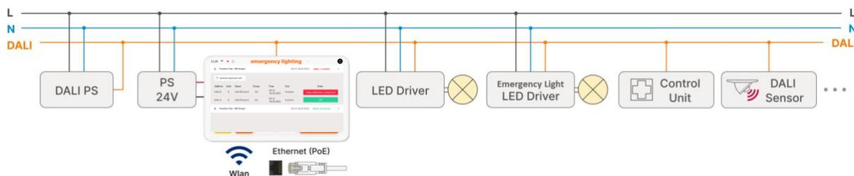
Figure 1 Typical Application – mixed DALI system
