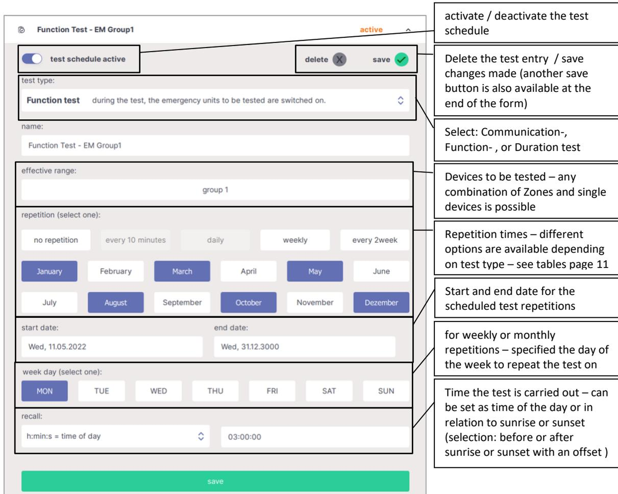
Figure 10 Configuration of emergency test schedules
