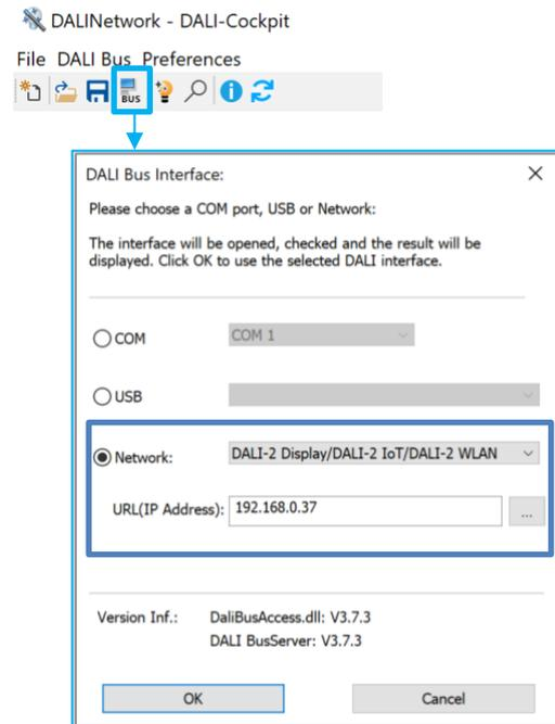
Figure 14 DALI Cockpit – selection of DALI bus interface
