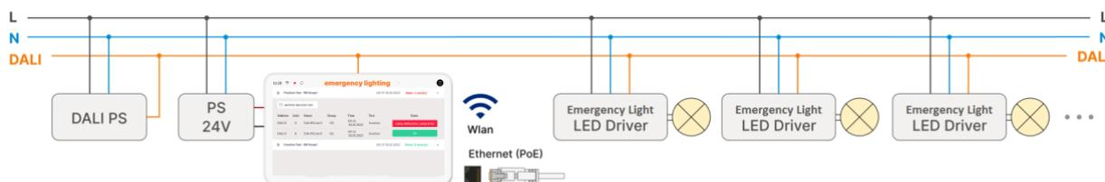
Figure 2 Typical Application 2 – Emergency light exclusive DALI system
