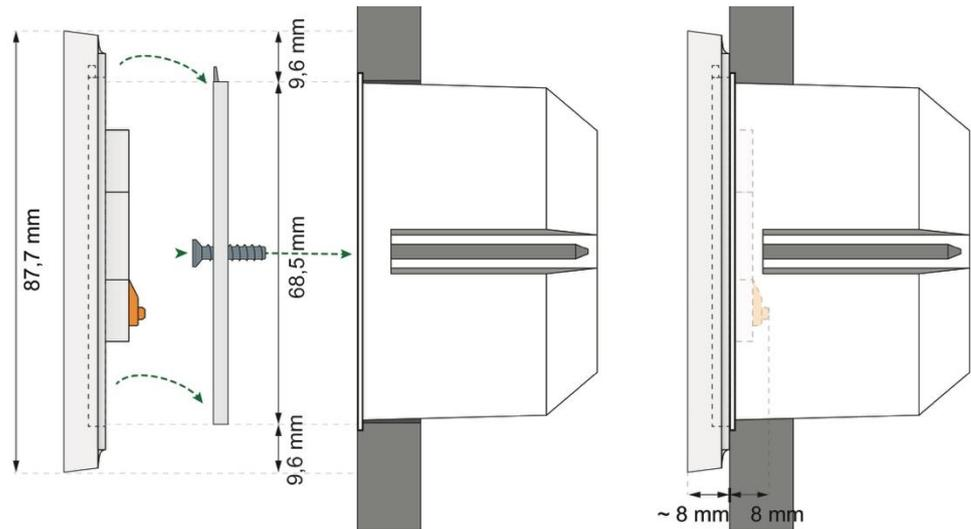
Figure 1 Installation: DALI-2 Touchpanel
