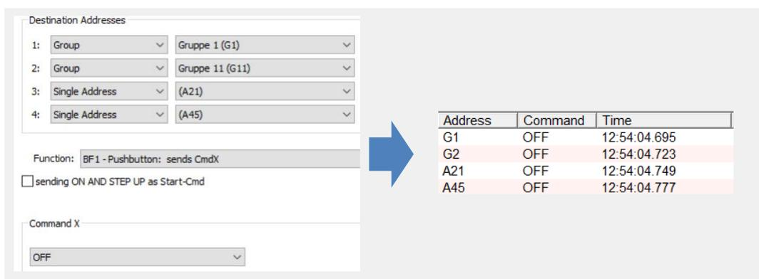
Figure 10 Example: Addressing Inputs 1-4 – sequentially processed
