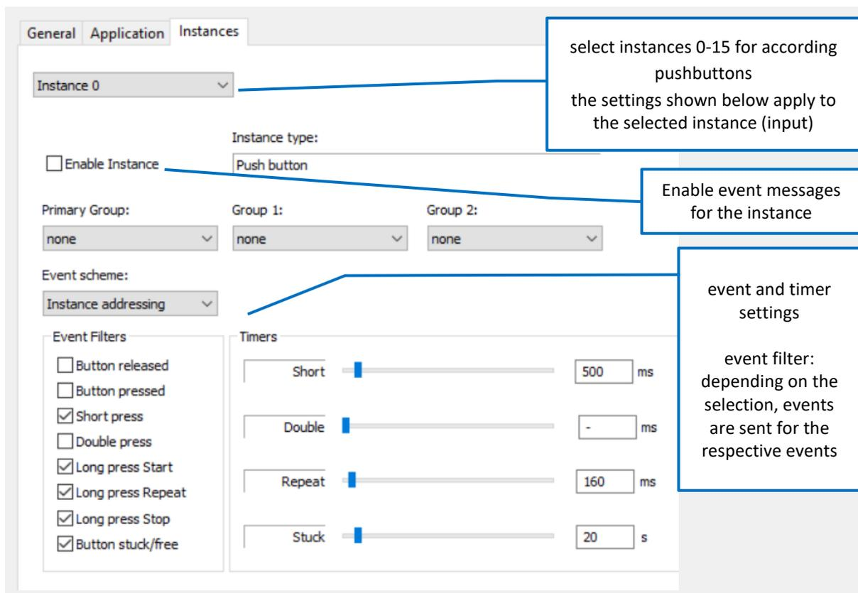
Figure 15 Instance Settings – Pushbutton Instances 0-15
