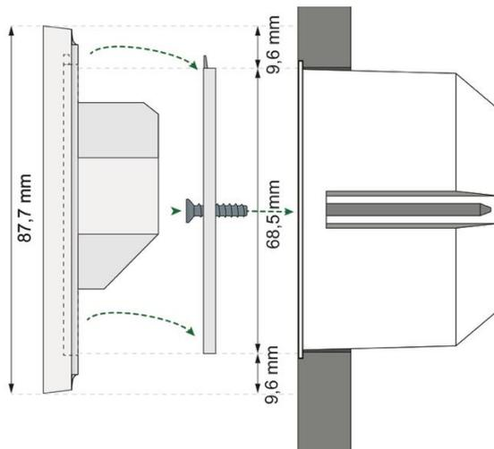
Figure 3 Installation DALI-2 Touchpanel PS
